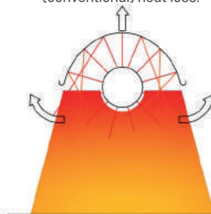
Classic parabolic reflector 25% convection (conventional) heat loss.
